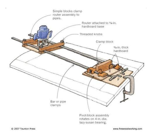
While building a gate, I was left with one major task—cutting an arch at the top. The thickness of the wood (8/4 mahogany) demanded a circle-cutting fixture that was very stiff and accurate. So I devised this fixture based on the 8-ft.-long pipe clamps I had used to glue up the gate. It consists of two bar or pipe clamps, a pivot-block assembly, and a router base. The clamp block on the pivot assembly is sized so that the pipes remain parallel from one end to the other.
